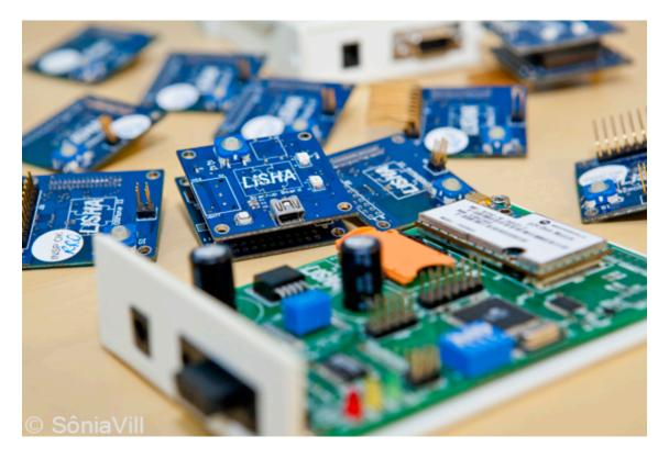
Within the CIA<sup>2</sup> project, LISHA and UnB are responsible for building an infrastructure for the Internet of Things (IoT). This infrastructure is comprised by an embedded platform (mote) and a no-legacy network stack. The network stack will focus on low resource utilization (including processing, memory, energy and communication bandwidth), while dealing with the platform's heterogeneity, mobility, noisy communication channel, scalability, and configurability.
