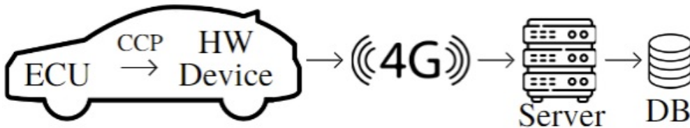
Figure 6 MAIN PARTS OF THE COMMUNICATION STRUCTURE
